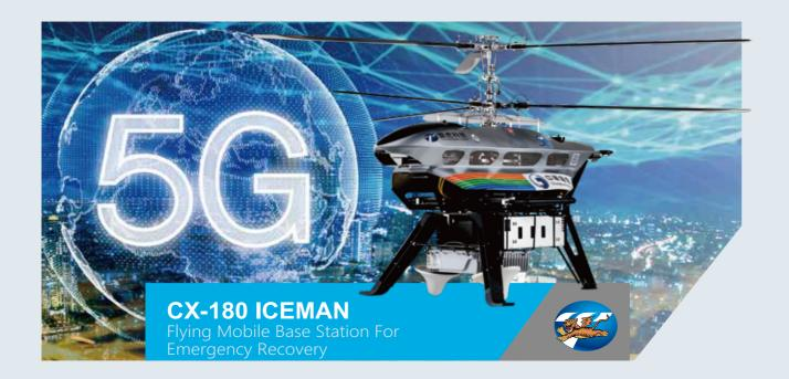
Thunder Tiger CX-180 ICEMAN is a collaboration project between Thunder Tiger and Chunghwa Telecom. The CX-180 helicopter is a flying 4G/5G Mobile Base Station equipped with small cells and antennas and can be easily transported, deployed, and moved quickly to accommodate rapidly changing conditions in emergency situations.
