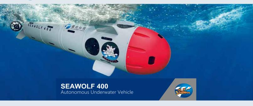
The Seawolf 400, an Autonomous Underwater Vehicle (AUV), is a MINI Cooper size submarine, designed to accommodate civilian and military applications, spanning from surveillance and strike capabilities to supporting environmental preservation and scientific exploration. It supports underwater missions up to 200m depths. In the development of our prototypes, we prioritize open architectures and modularity to streamline the integration of sensors and facilitate future upgrades.
