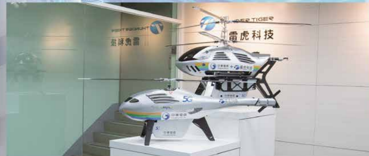
• Thunder Tiger flying mobile base station for emergency recovery CO-ENGINEERED with Chunghwa Telecom
